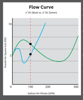
For our example, the is designing their water use at a nominal flow rate of 100 gpm (gallons per As shown in the figure, the pressure loss of the two-inch
